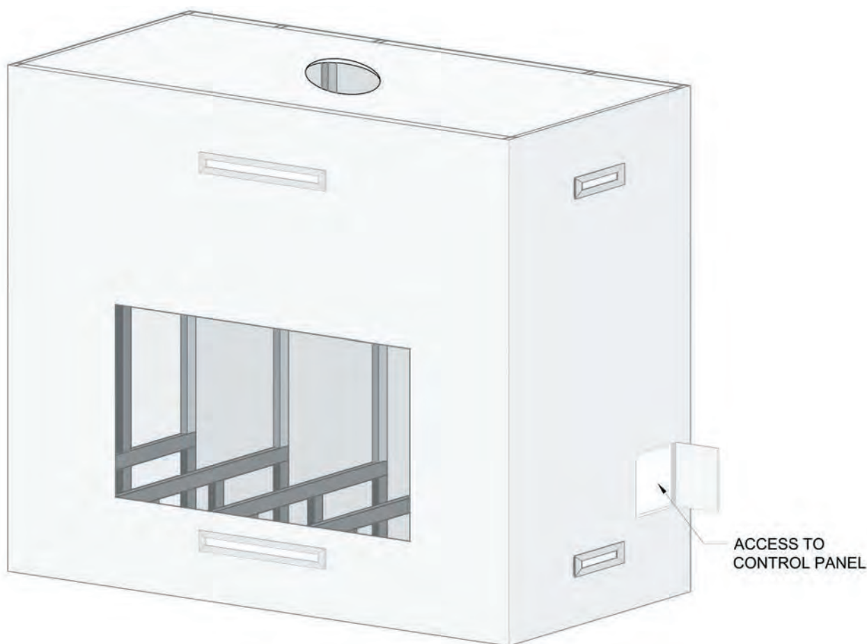
Figure 1.5 (Control panel location)
